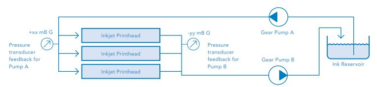
Figure 1. Ink Supply System for Recirculating Inkjet Printheads
