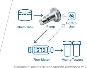
Micropump pumps deliver smooth, controlled flow of whitening agents to the bleaching towers.
