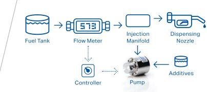
Micropump pumps deliver smooth, controlled flows of fuel additive into a fuel dispensing system.
