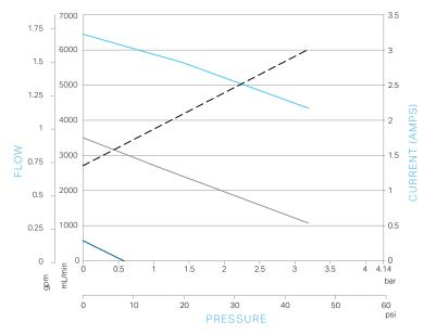
FLOW RATE NOMINAL: 2700 mL/min (@ 1.4 Bar, 3V) FLOW RATE MAX: 6435 mL/min (@ 0 Bar, 5V) DISPLACEMENT: 1.17 mL/rev
