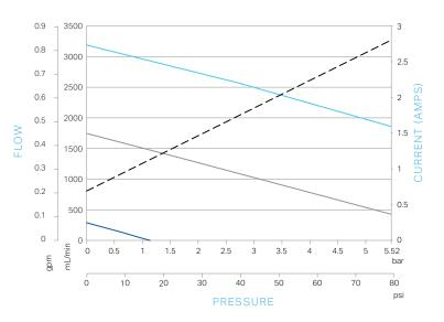
FLOW RATE NOMINAL: 1000 mL/min (@ 2.8 Bar, 3V) FLOW RATE MAX: 3190 mL/min (@ 0 Bar, 5V) DISPLACEMENT: 0.58 mL/rev
