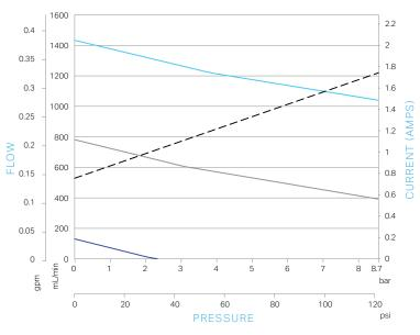
FLOW RATE NOMINAL: 550 mL/min (@ 4.3 Bar, 3V) FLOW RATE MAX: 1430mL/min (@ 0 Bar, 5V) DISPLACEMENT: 0.26 mL/rev
